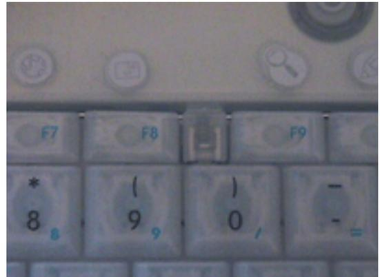
Apple has made access to the internal components easier than ever. There are two small latches on the keyboard, located between the sets of function keys. When unlatched, the keyboard lifts up, revealing the hard drive, AirPort card, RAM, and CD drive. You can easily add RAM—there's even a diagram printed inside showing you how to do it! There really isn't access to anything else, and it would void your warranty anyway if you opened it up any more.
