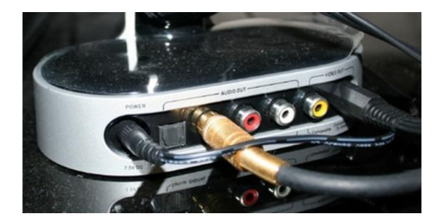
My TOSLINK cable disappeared in a recent move, so I was unable to test the optical digital output of the i-20 in time for this review. The coaxial digital output (using a conventional RCA cable) works a treat, without any analog hiss at all, and, barring the re-appearance of that missing TOSLINK cable, is my current method of choice for connecting the i-20 to my receiver.
