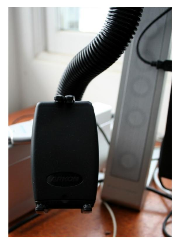
At the other end is a flat plate with four movable "fingers" on it. The bottom portion of the plate is on a spring-loaded slide, allowing the Raptor to hang onto any small electronic device up to about the height of an iPhone in a typical case (about 5'').
