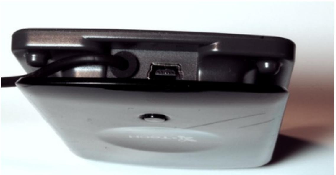
The cable management doesn't play nice with the USB charging port. As you can see here, the port is easily buried under the SolarCharger's power cable.
