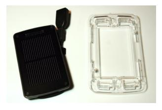
The frame is removable if you want to save space or weight, but it's an essential accessory if you want to mount the SolarCharger on a window. The suction cups attach to the holes in the frame.
