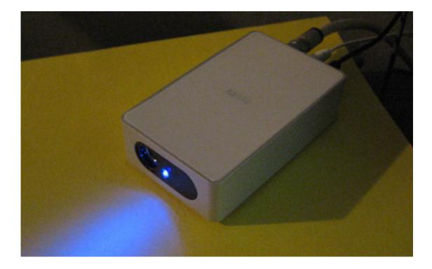
The EyeTV 250 hardware unit isn't just a converter box to let data flow through a coax cable into a Mac's USB port. The device also contains a compression chip which converts the incoming data into MPEG-1 or MPEG-2 format. Sure, my computer could do that, but it'd be highly processor-intensive. Since the EyeTV 250 is doing the heavy lifting, "older" computers (like my two-year-old PowerBook G4) can be used to watch and record TV.
