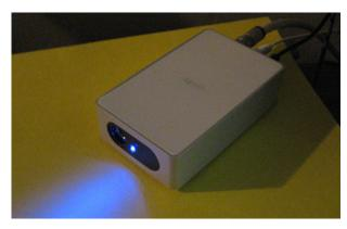
The EyeTV 250 hardware unit isn't just a converter box to let data flow through a coax cable into a Mac's USB port. The device also contains a compression chip which converts the incoming data into MPEG-1 or MPEG-2 format. Sure, my computer could do that, but it'd be highly processor-intensive. Since the EyeTV 250 is doing the heavy lifting, "older" computers (like my two-year-old PowerBook G4) can be used to watch and record TV.
